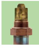
State of oxygen sensor: Greenish, grainy discoloration.
