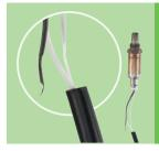
**State of oxygen sensor:** Broken cable.
