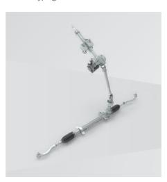
Servo unit on the steering column is specifically for vehicles with low steering effort: entry-level sub-compact to mid-sized vehicles.
