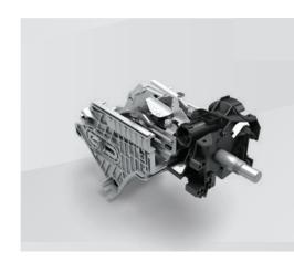
Connects the steering wheel with the steering shaft and offers a full adjustment of height and tilt for driver comfort.
